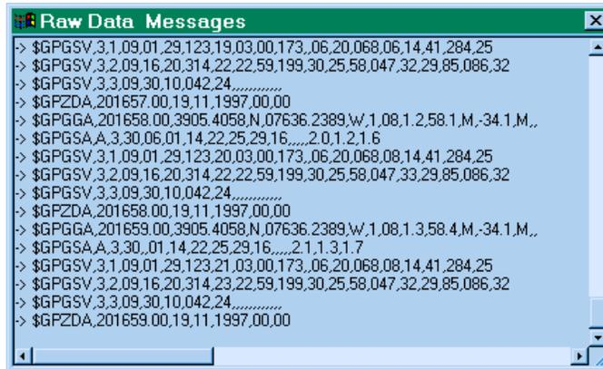
**NMEA data:** The sample window, above, shows raw NMEA data from a GPS receiver (in this case a Motorola Oncore). The NMEA data begins with the \$ character. The characters preceding the data on the line are special in that they are added by Tac32Plus to provide basic status information.
