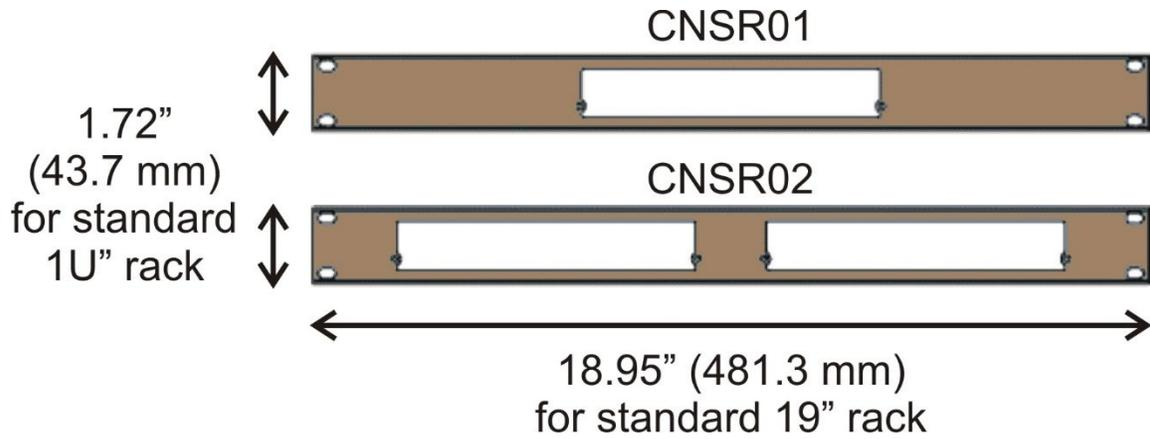
The CNS Clock II is installed into the rack panel as shown below. Mount the panel to the rack with spacers shipped taped to the rear of the rack panel.
