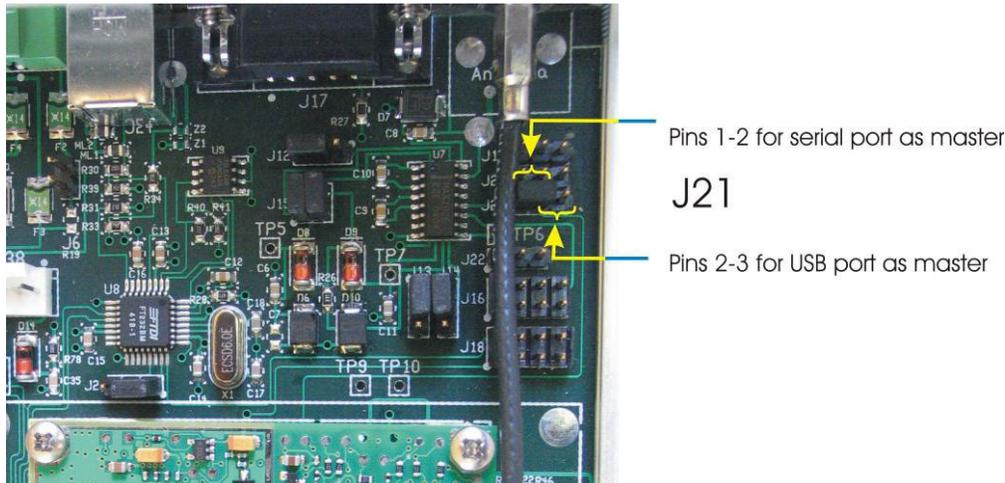
For all other boards the default is that the USB port automatically becomes the master over the RS-232 port when the CNS Clock II senses an active USB port and no jumper needs to be changed. In the event that you wish to force either the USB or RS-232 port to be the master all the time, change the jumper J21 on revision C or J24 on revision D and later boards as shown in the chart at the beginning of this section.
