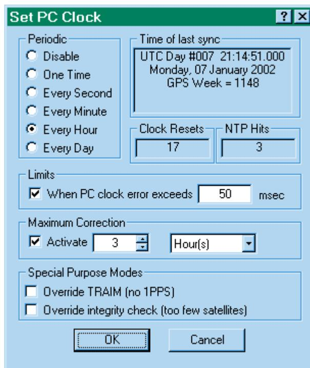
**Every Second:** Setting the clock every second has the advantage of minimizing the long-term drift in the computer's clock at the cost of some short-term jitter.
