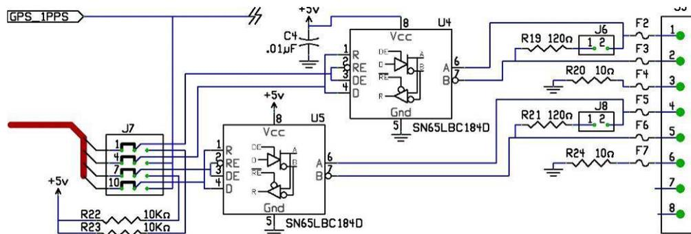
**Signals:** The CNS Clock II with the RS-485 RFID time code option provides two outputs at the rear panel, a jumper selectable output (pins 1-2-3), and a 1PPS signal (pins 4-5-6). The jumper selectable output period ranges from 2 milliseconds to 250 milliseconds, settable to values indicated in the table below.
