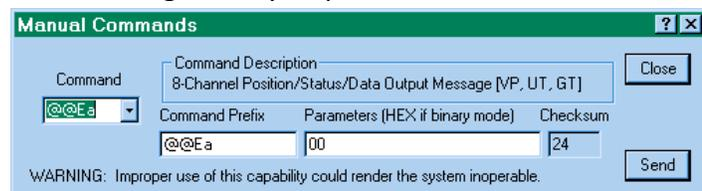
**Command:** Use the drop-down arrow at the right edge of this control to see a list of the standard commands for the GPS receiver. The command list is mode sensitive so it will show a
