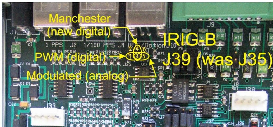
There must be no more than one jumper on the terminal block.
