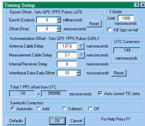
For high accuracy timing synchronized to UTC the Epoch, Offset and Intentional Early Offset controls are normally set to zero (0) and the Antenna Cable Delay, Measurement Cable Delay and Internal Receiver Delay controls are set as accurately as possible.
