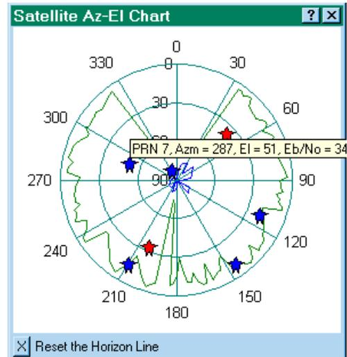
Similarly, there is a blue line in the center of the plot that represents the "hole in the sky". This is the area directly above the station location where no satellites have been tracked. This area is larger for stations close to the North or South Pole and diminishes to nothing at lower latitudes.
