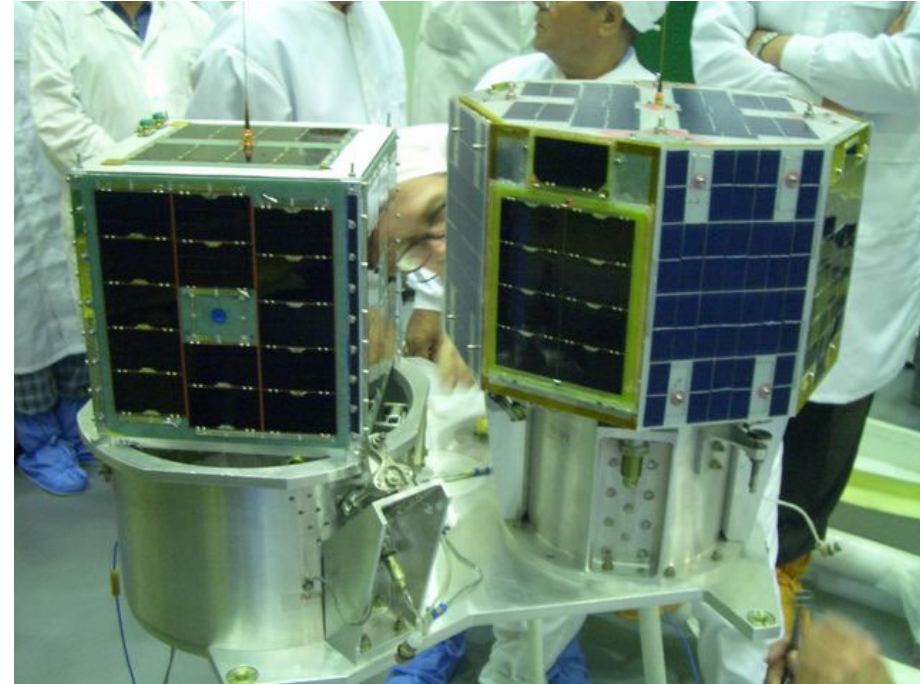
Echo (left) with UniSat-3 mounted on dispenser plate
