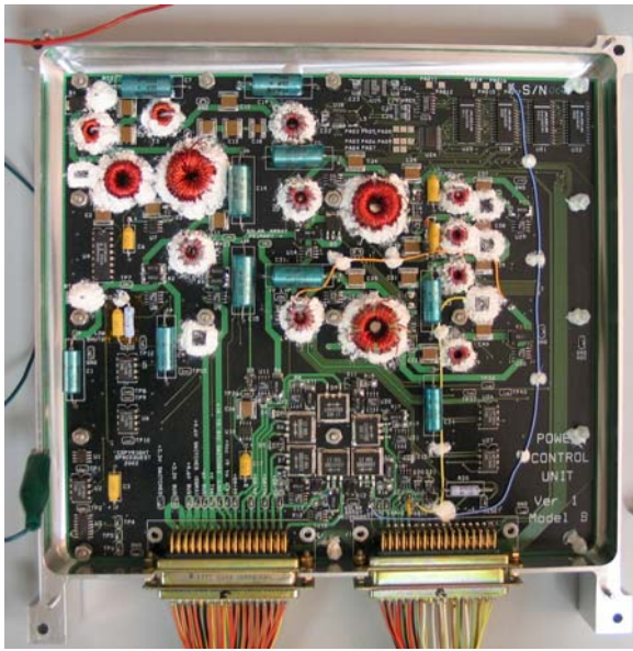
Figure 13: Battery Control Regulator
