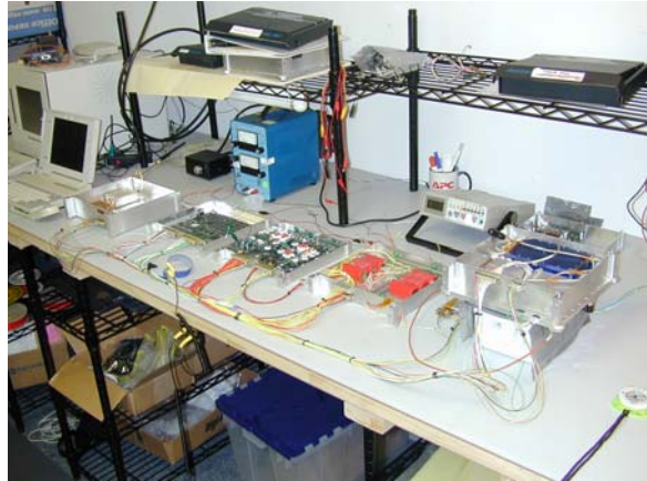
Figure 3: Echo flight hardware powered up for testing in "flat-sat" configuration
