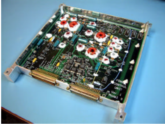
Figure 10: Battery Control Regulator
